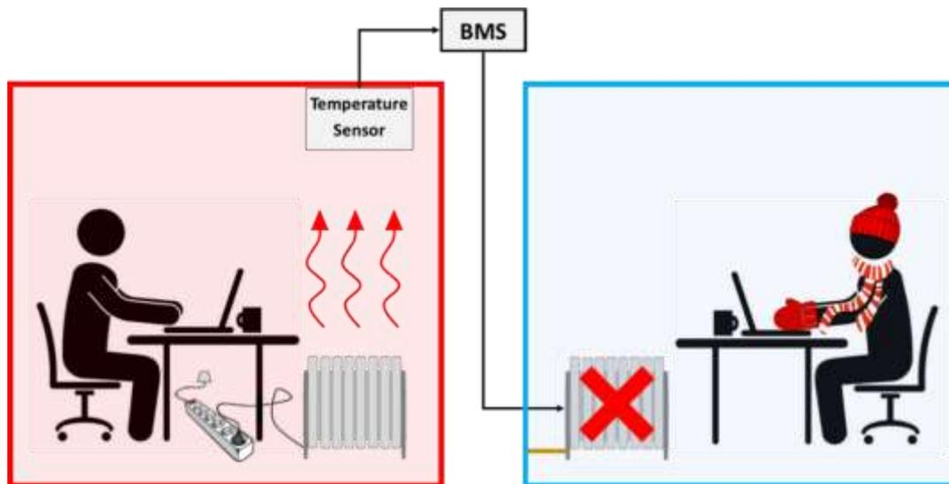
Figure 1: Impact of supplementary electric heaters on the BMS, and wider building heating system
